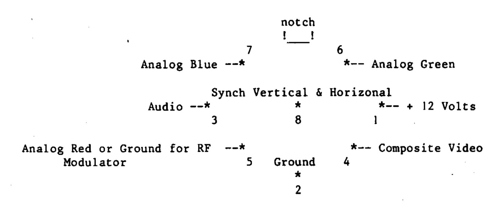
Video Output Control Pins and Jumper
